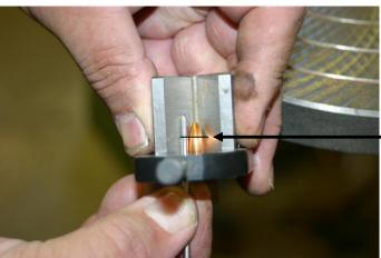
Compare the refill to the lead nib. Flip the lead over and drill with 9/64 to about 3/16 before exit out the small tip.
