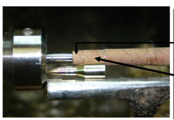
After rounding the blanks, mark critical areas to help guide next turning.
