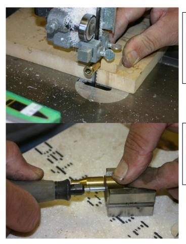
Cutting the brass on the band saw works. I use a blade that is too dull for wood. Hate to change blades so I don't use the band saw very often. However the brass is cut, some cleanup is needed to remove burrs. This will become evident as you make these pens. Just be careful. Sanding scars the brass and the
