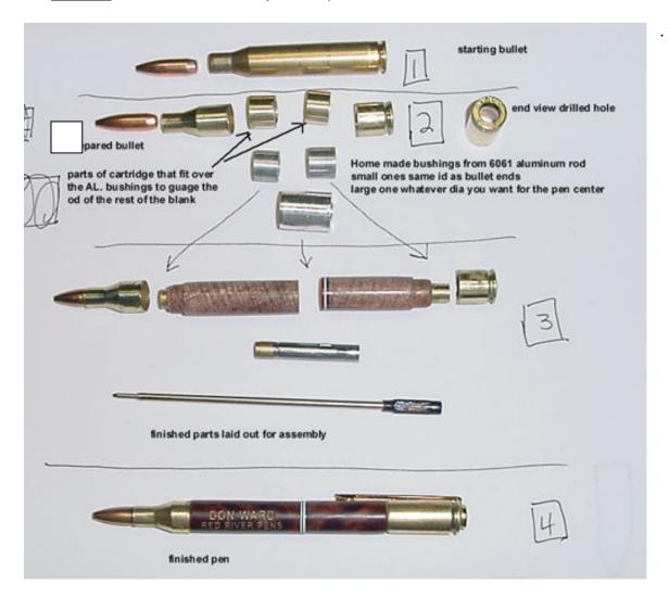
Not a necessity, but powdercoating the brass parts with clear powdercoating paint makes them retain their polished shine. The brass will never tarnish under this stuff. It is tougher than woodpecker lips.
