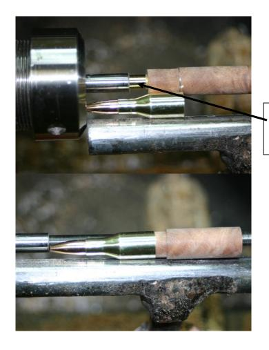
End of brass tube needs to be removed so it doesn't hit the end of the lead bullet.
