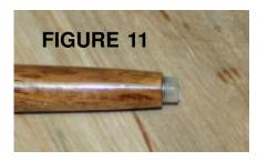
Figure 11 shows the mechanism protruding through. Test often and make sure the metal tip will screw on and tighten against the wood. See next figure.
