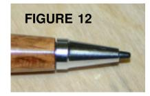
If too much wood is removed the metal tip will bottom out before meeting the wood and the tip and mechanism moves in and out. It does not seem to affect the use of the pen but neither does it show off my turning skills, if in fact I have any skills. Take it slow; remove a little at a time and check for fit often.
