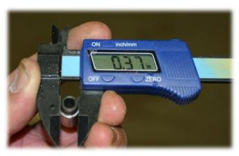
Measure the real bushing for future reference. This is the end that will go inside the brass tube from the pen kit. I've chosen to make sierra bushings for this tutorial.
