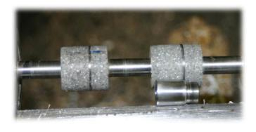
I have the two blanks mounted with slimline bushings to separate them. I've marked the blanks to indicate the two diameters. The right side will go inside the tubes and the left side will be the diameter of the finished blank, or at least the guide for the finished pen.
