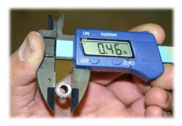
Measure the other end of the bushing. This end is the pen diameter end.
