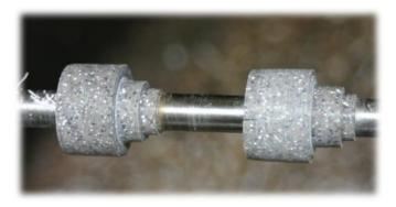
I used a parting tool to get the right end of the bushings close to final dimension. I turned a small section to almost finished size.
