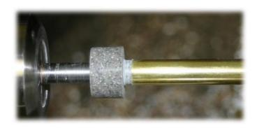
I then removed one of the partially made bushings and placed the sierra tube over the slimline bushings. I used sandpaper to get the final size of the bushing to insert inside the tube. The tube is used to find the correct size.
