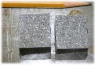
Look Ma, no visible seams. If corian is glued together correctly, the seams will be invisible. I sand the mating surfaces lightly.
