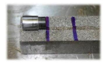
Mark the bushings lengths using real bushings if available. If not, then choose a length for the bushing.
