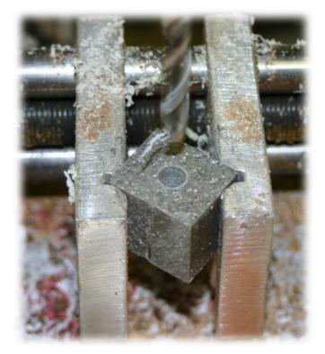
Drill the bushing pieces with 1/4 inch to fit the mandrel or drill with 7mm and glue in a brass tube. I choose to drill 7mm and use a tube. It isn't necessary, but I do use a tube.
