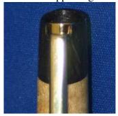
**Figure 6**I use a drimmel tool to cut the notch for the clip and light sanding to remove the rough edges. The notch can be cut before the finish is added. Also, using a black sharpie inside the 11/32
