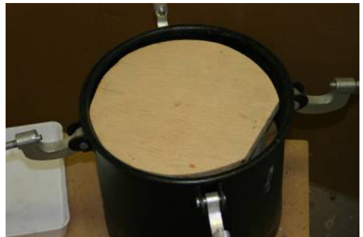
Racks and molds are in the tank. It is time for the lid and pressure.
